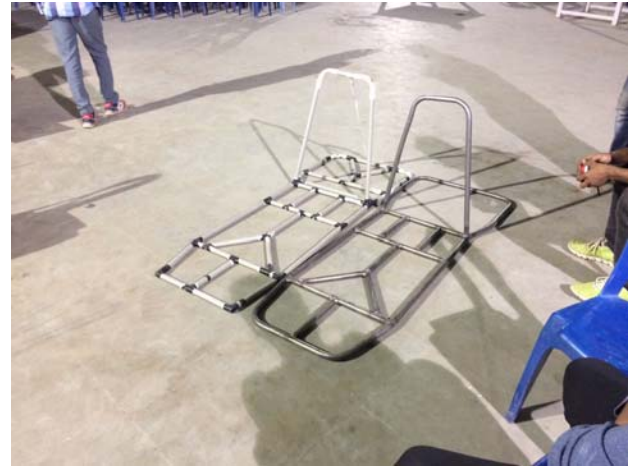
Figure 15. A prototype PVC model and an actual chassis made by the material AISI 4130 kept side by side.
